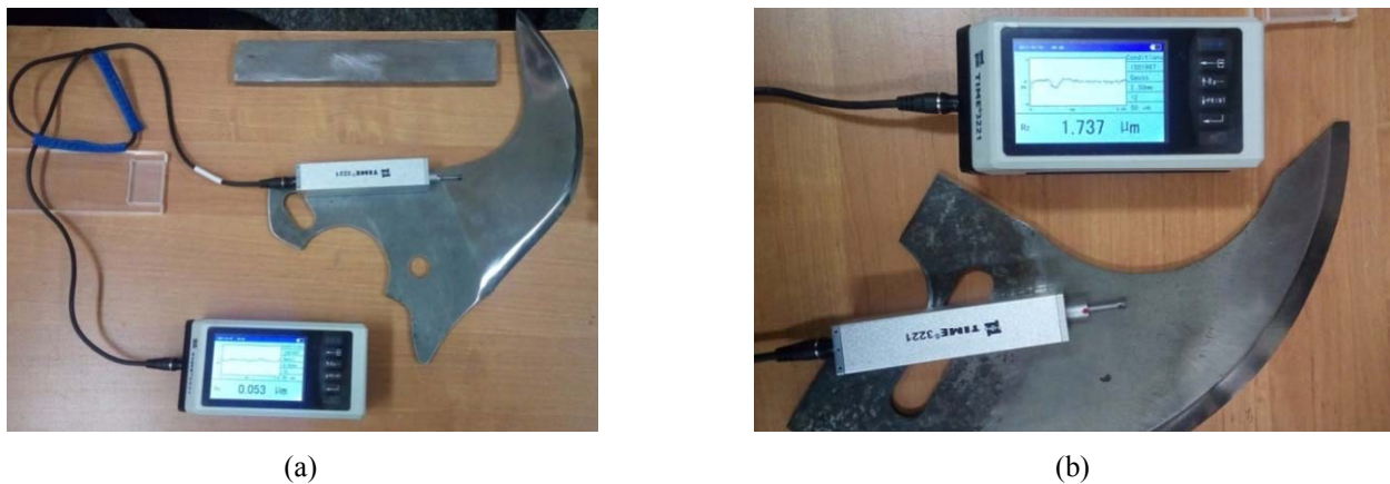
Fig. 8. Measurement of the roughness of the knife surface using a TIME 3221 profilometer: (a) the knife of the Laska KR-330-2V cutter; (b) the knife of the L5-FKB cutter.
