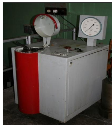
Fig. 2. High pressure plant (hydrostat).
